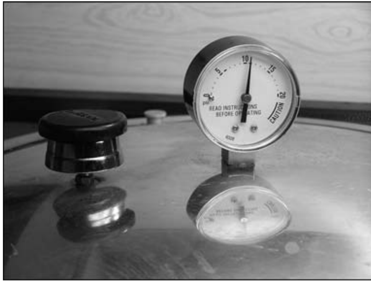
The pressure canner is working—here the dial gauge shows just over 10 pounds of pressure. (Photo courtesy of Daniel Gasteiger)
